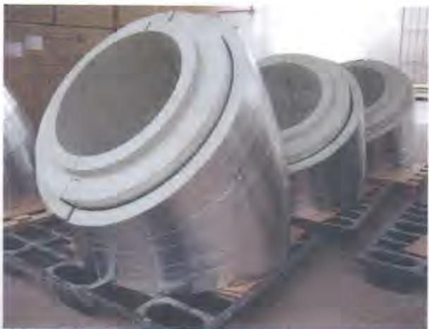
Figure 6. Prefabricated elbows with Tembutil-IF.
